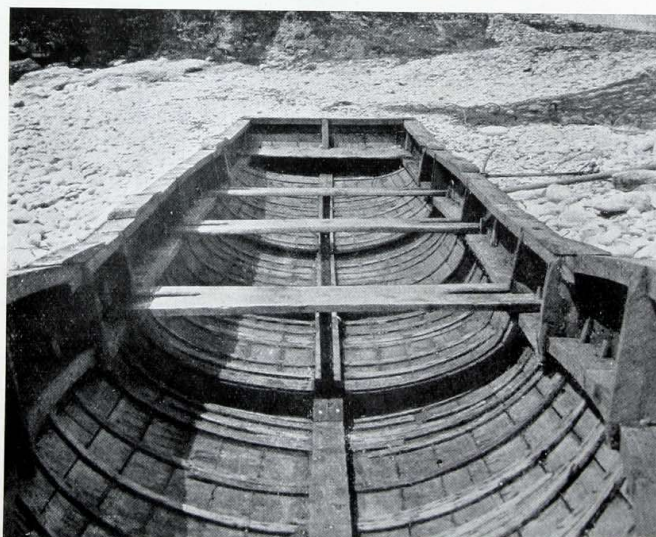
FIG. 3. INTERIOR OF AN ACHIL ISLAND CURRAGH, LOOKING AFT
